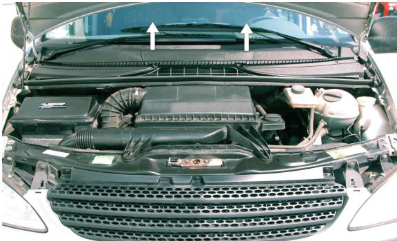
(EN) Remove the segment of the screen under the windshield
